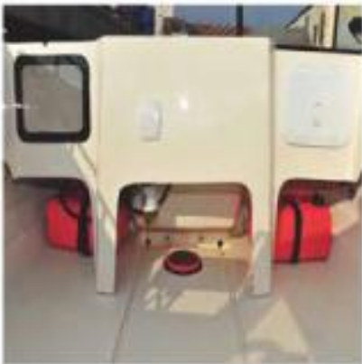
Twin 25-litre fuel tanks held in place by straps gives a very useful range. Built in livebait tank with aerator as standard
