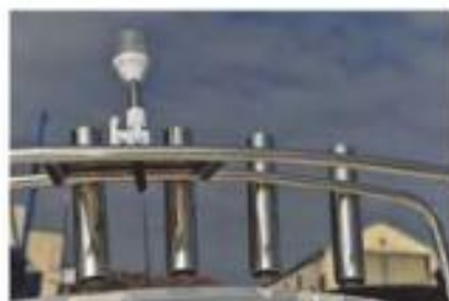
Coachroof hardware supports lighting, antennae and rod holders
